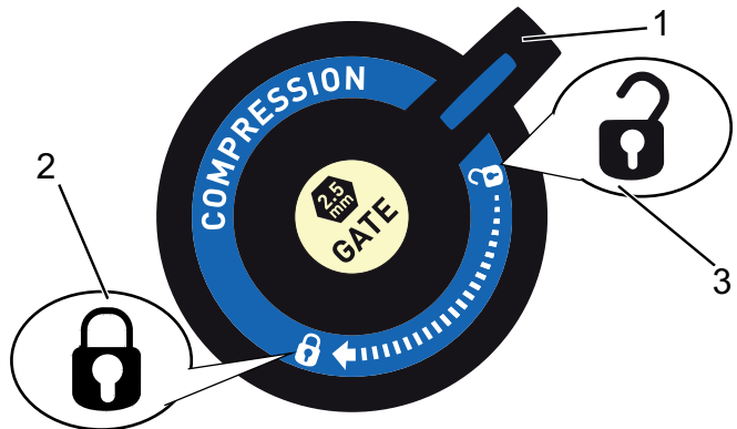
Figure 30: Fork lock with locking lever (1), which can be placed in the closed (2) or opened (3) position
