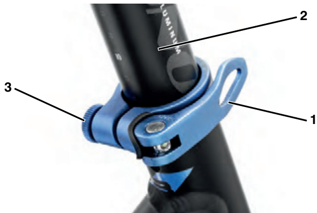
Figure 18: Seat post (2) quick release in the clamping lever end position on the seat post (1) and its knurled nut (3)
