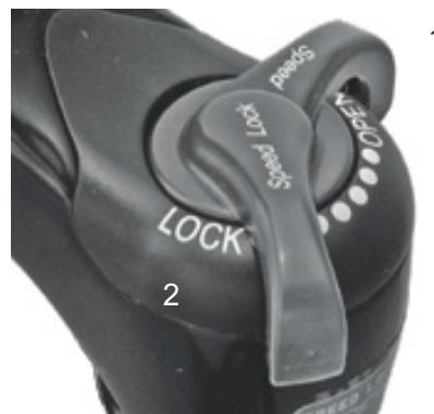
Figure 74: Suntour compression adjuster with the OPEN (1) and LOCK (2) positions
