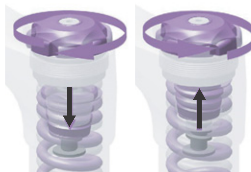
Figure 52: Screwing and unscrewing the pre-tension adjustment ring.
