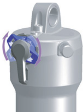
Figure 65: Changing compression adjuster to a harder setting
