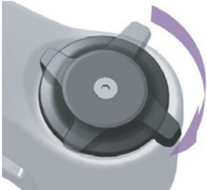
Figure 89: Changing compression adjuster to a harder setting
