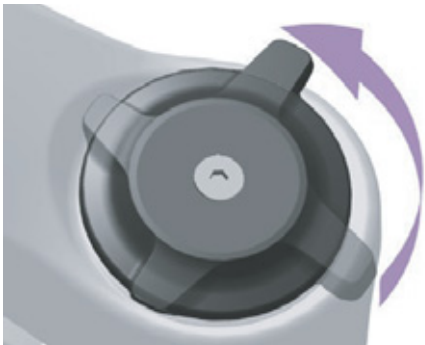
Figure 90: Changing compression adjuster to a softer setting
