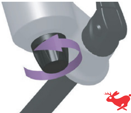
Figure 102: Turning rebound damper towards hare symbol
