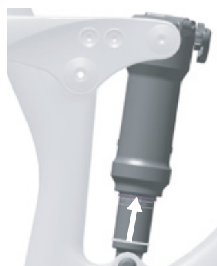
Figure 57: Moving the O-ring on the rear frame damper
