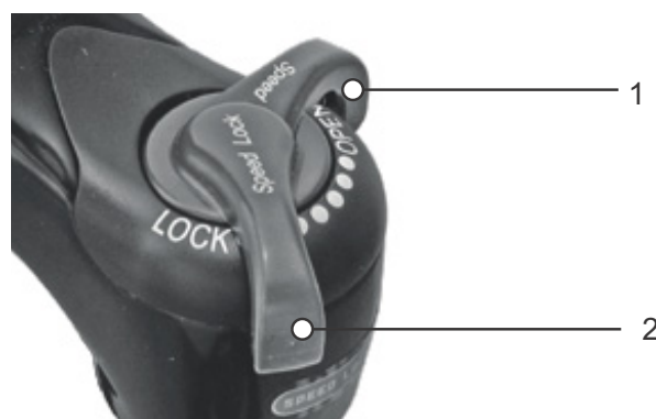
Figure 88: Suntour compression adjuster in open (1) and closed (2) position
