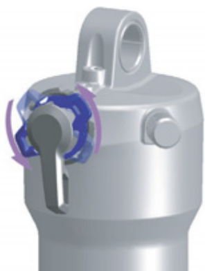
Figure 66: Changing compression adjuster to a softer setting
