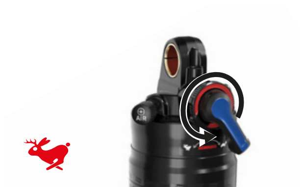
Figure 62: Increasing the rebound speed
