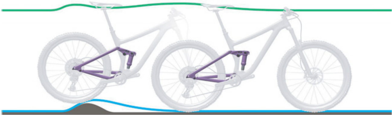
Figure 113: Excessively hard damping in the rear frame damper on bumps
