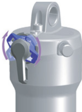
Figure 112: Changing compression adjuster to a harder setting
