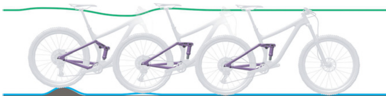
Figure 107: Rear frame damper rebounding too quickly
