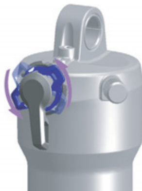
Figure 114: Changing compression adjuster to a softer setting
