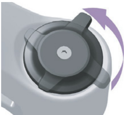
Figure 106: Changing compression adjuster to a softer setting
