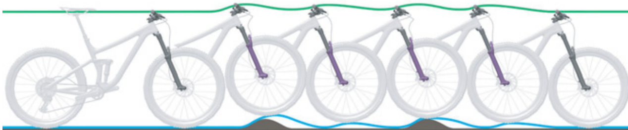
Figure 99: Suspension fork rebounding too quickly
