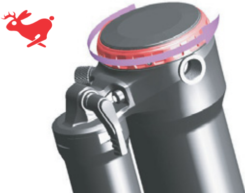
Figure 110: Turning rebound damper towards hare symbol
