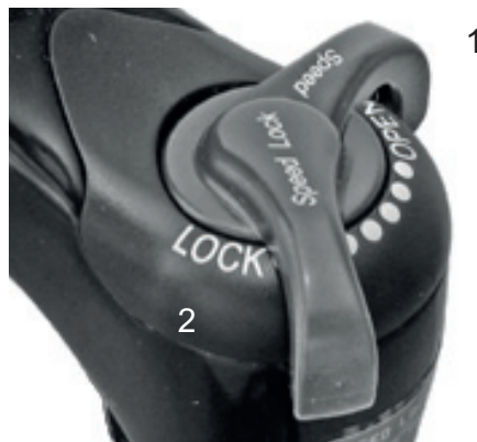
Figure 63: Suntour compression adjuster with the OPEN (1) and LOCK (2) positions
