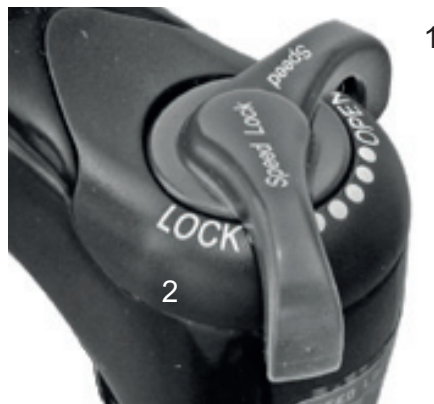
Figure 50: Suntour compression adjuster with the OPEN (1) and LOCK (2) positions
