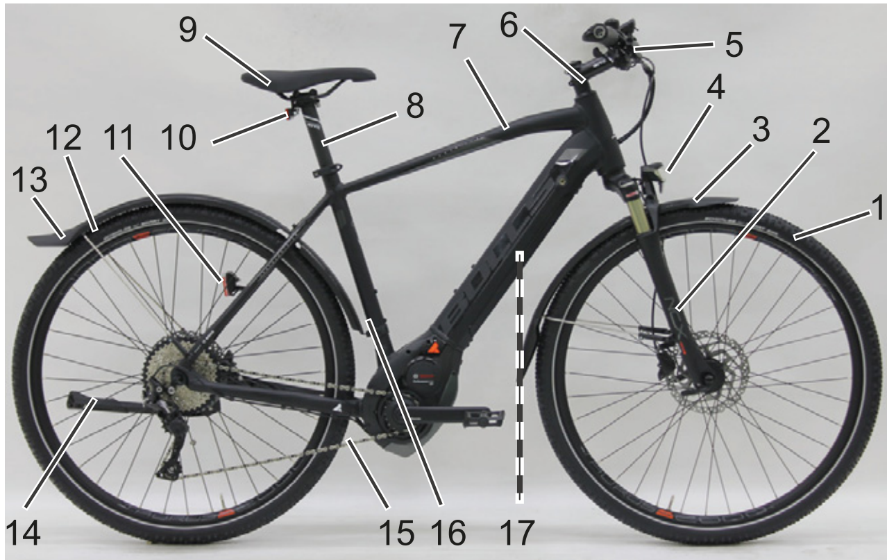
Figure 2: Pedelec viewed from right, Bull Cross Rider used as example
