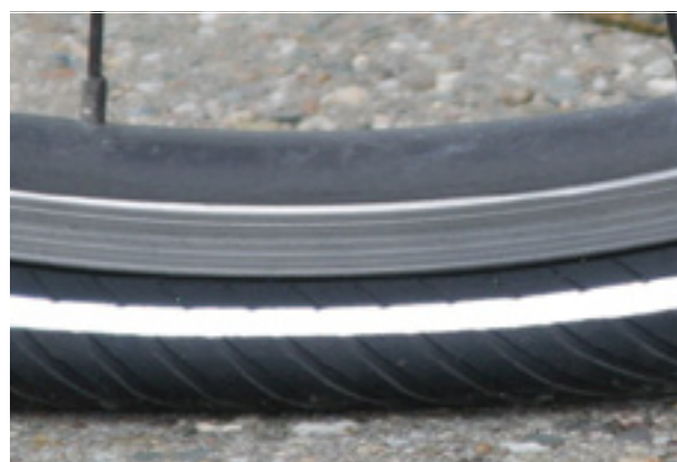
Illustration 103 : Pression largement insuffisante
