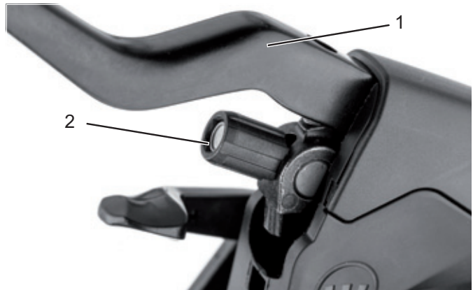
Figure 73: Brake lever (1) of the hydraulically operated rim brake with setting bolt (2)
