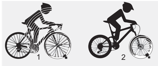
Figure 7: Bicycle without suspension (1) and with suspension (2) when riding over an obstacle
