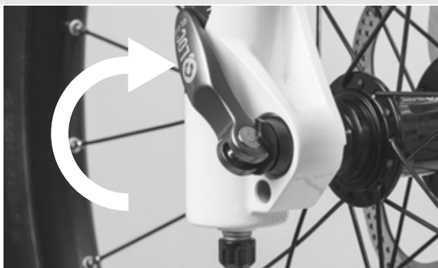
Figure 38: Closing the quick release
