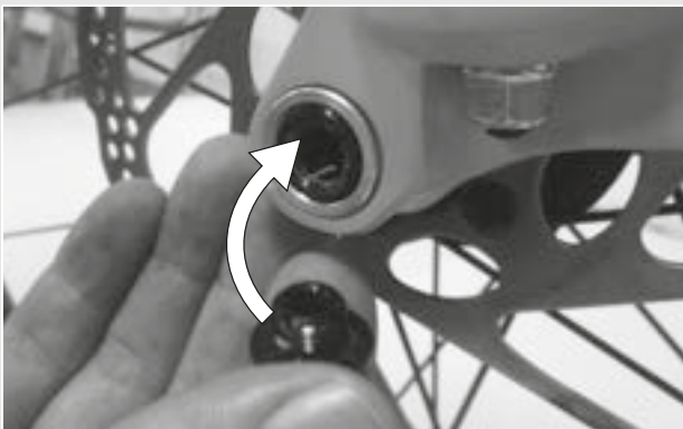
Figure 25: Pushing the quick release lever into the axle
