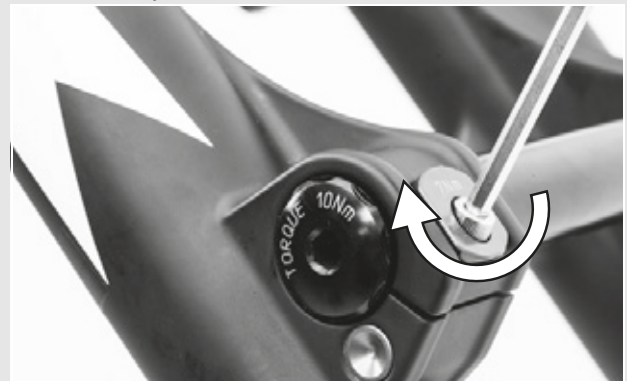
Figure 28: Tightening the axle
