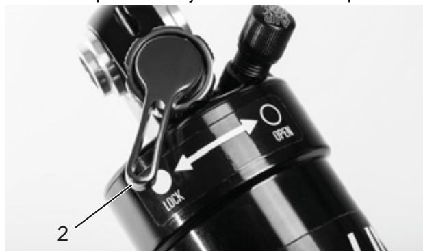
Figure 76: Suntour compression adjuster closed (2)
