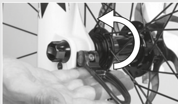
Figure 32: Securing the lever
