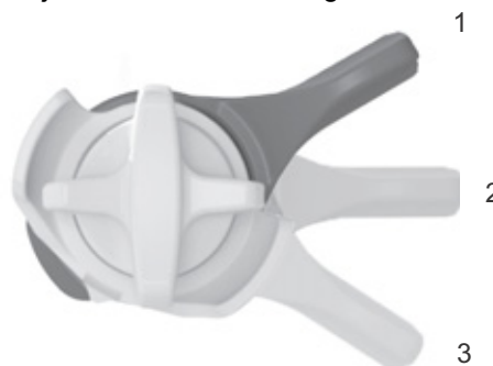
Figure 73: FOX compression adjuster on the rear frame damper with the OPEN (1), MEDIUM (2) and HARD (3) positions
