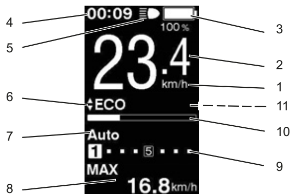
Figure 19: On-screen indicators overview
