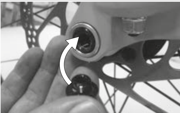
Figure 26: Pushing the quick release lever into the axle
