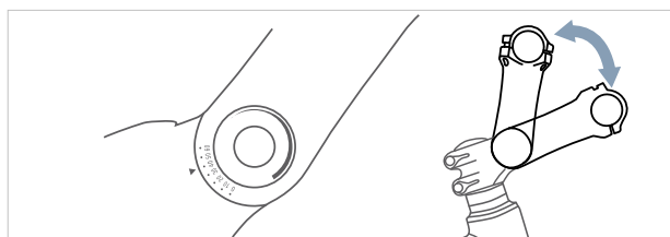
Figure 28: Different versions of angle-adjustable stems
