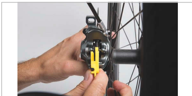
Figure 51: Checking the brake lining when fitted with the help of the transport lock
