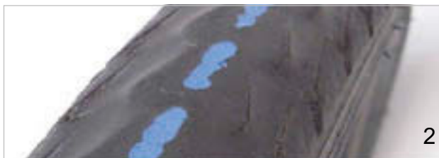
Figure 49: Tyres without a tread which can be replaced (1) and tyres with puncture protection showing through (2) must be replaced
