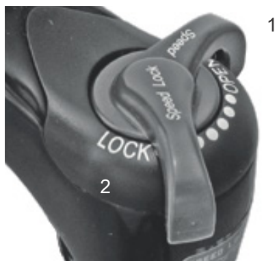
Figure 32: Suntour compression adjuster with OPEN (1) and LOCK (2) positions
