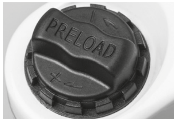
Figure 26: Negative deflection setting wheel on the suspension fork crown
