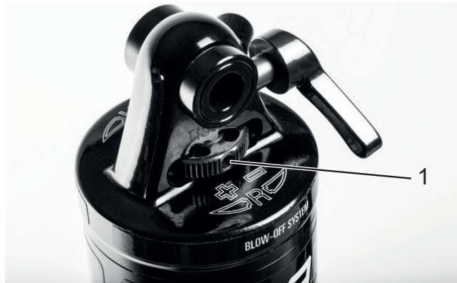
Figure 53: Suntour rebound adjuster wheel (1) on the rear frame damper
